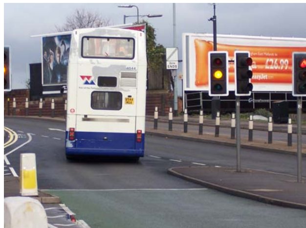
A bus gate in operation: as the bus approaches, the lights change to give the bus priority
