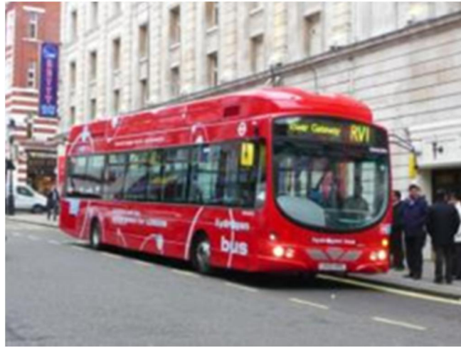
Figure A1.10 Wrights Pulsar fuel cell hydrogen/electric
