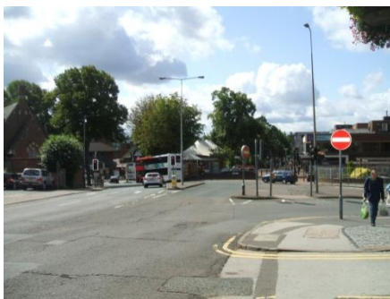
Large junction space and wide carriageway through an area where place should be prioritised, with several key desire lines severed by the wide highway space, leaving the place centre as an island and fragmenting the place.
