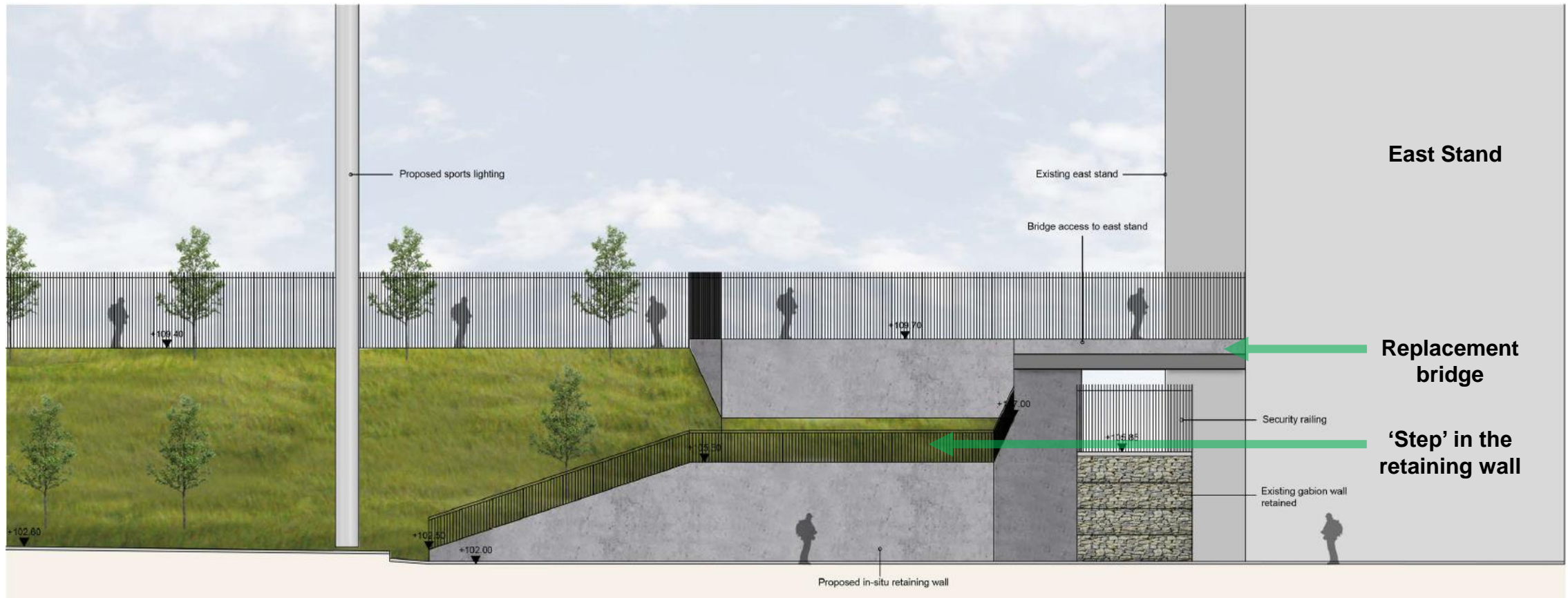
An image showing the replacement bridge and updated design of the East Stand South Retaining Wall
