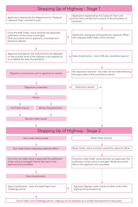
Diagram: Section 247 procedure
